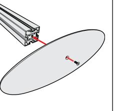
**Base Plate & Extrusion Connection**
